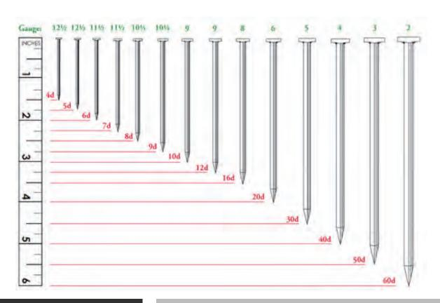
Material Low Carbon Steel/Medium Carbon Steel
